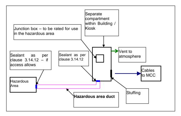
Ducts leaving a hazardous area or a Severn Trent Zone BZ and delivering cables to a junction box or a kiosk on a stand shall be sealed as they exit the ground; cables are required to pass through a minimum unobstructed air gap of 300 mm before entering the enclosure.
