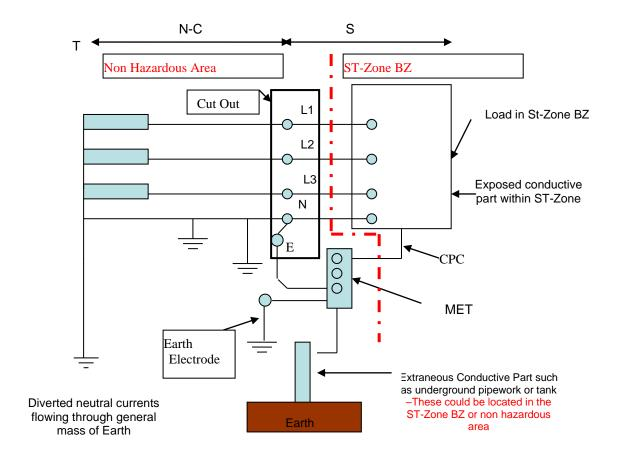
**F.3.4.6.2** Generator Connection facilities – an earth electrode system (which must be switchable) is required as part of the electrical installation. It shall be designed to be utilised for this purpose and for earthing of the hazardous area.
