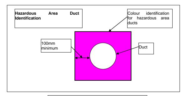
Hazardous Area Duct Duct Sealing System to be retained at all times
