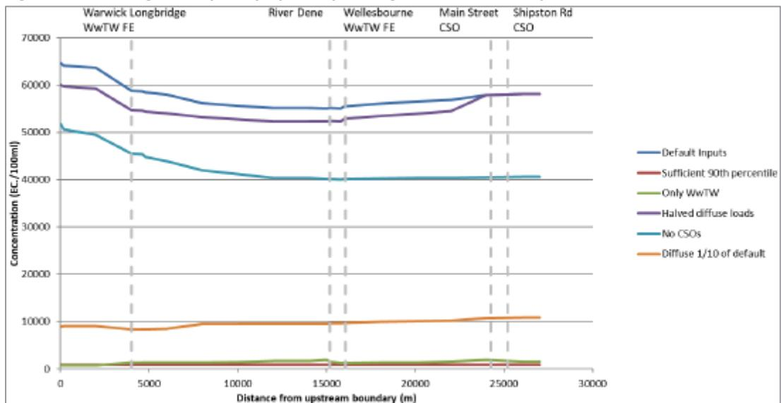
To assess which **storm overflows** require intervention we produced storm overflow spill volumes using our calibrated sewer hydraulic models. For this initial assessment, we used the 1-in-1-year events. Whilst it is likely that a small number of spill events per year will not prevent us from achieving our desired outcome, we have used the worst-case 1-in-1-year event as an allowance for the future impact of climate change, growth and urban creep.
