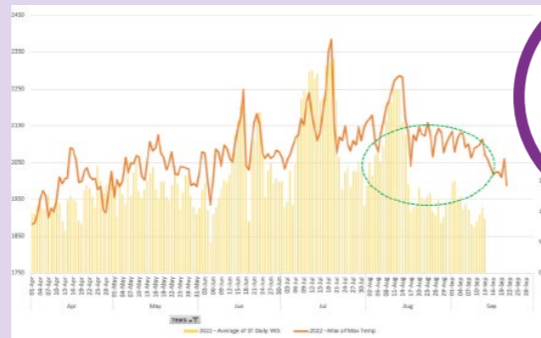
Graph showing the relationship between high temperature (in orange) and water demand (in yellow) in 2022, highlighting the success of our customer campaign in reducing demand (in green).
